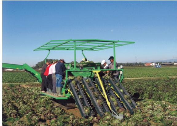
Rapid SR is a machine for head vegetables harvest. The harvesting element is equipped with two vertical corrugated belts that allow to transport tightly the product and with an inferior belt that carries the product to an upper belt that is to say a work surface for the cleaning.
