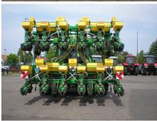
SIGMA 5 is a pneumatic single seed precision seeder for seeding on semi no tilled soils. With solid quality construction, combining simplicity, versatility and reliability in seeding even at speeds of up to 10 / 12 km/h. The double disc wheel traction assures a constant depth seeding even in extremely difficult conditions.
