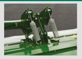
Most rear mowers have a central pin which allows the mower to move left and right to adjust to changes in ground condition. The McHale Pro Glide is different in that it is fitted with a patented 3D ground tracking suspension unit, which allows the mower to:
