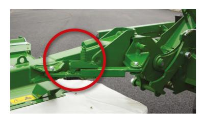
The Pro Glide rear suspension springs react instantly to ground contours, which results in a high quality cut even when working at high ground speeds. This allows the mower to easily mow on rough or undulating terrain and still deliver optimum results.
