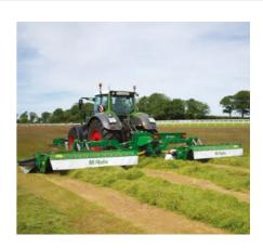
The Pro Glide range of rear mowers are fitted with patented ground adaption technology, which allows the bed to move back and up if the bed encounters small obstacles. This results in higher mowing speeds being able to be achieved without the interruption of having to reset the break back.
