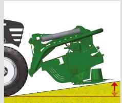
The Pro Glide front mower has its own independent suspension, which allows the mower to automatically move up & down independent of the tractor and has a vertical travel range of 500 mm. If mowing into a dip, the angle of the cutter bar will automatically adjust down and while mowing into an incline the cutterbar angle will automatically adjust up.
