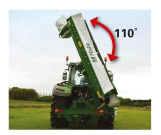
For transportation, the McHale Pro Glide folds vertically to position itself behind the centre point of the tractor for safe transport. The transport height of the machine is reduced as the mower bed is at 110 degree angle.
