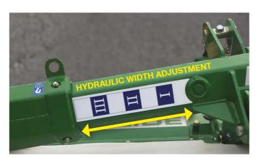
Hydraulic Width Adjustment is available as an optional extra on the McHale Pro Glide B9000 and the B9600 combination mowers.
