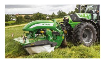
McHale's design team have designed the frame on the Pro Glide front mower to place the centre of gravity as close as possible to the tractor, which results in unrivalled responsiveness to changes in ground conditions.
